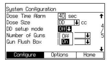
Fig. 55. Configure Screen 4, dynamic dosing setup mode enabled
